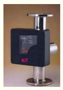
Metal Tube Rotameter is a variable area flowmeter Model KIT series is suitable for gas and liquid flow measurement even under high pressure and high temperature. Standard metal flow tube is in SS 316 and for corrosive applications the metal tube, orifice and float can be lined with PTFE. KIT series metal tube rotameter comes with optional limit switches and 4-20ma output.
